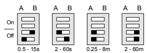
Switch positions shown above for the "Off period". The same positions are used for the "On period" (top two switches).
