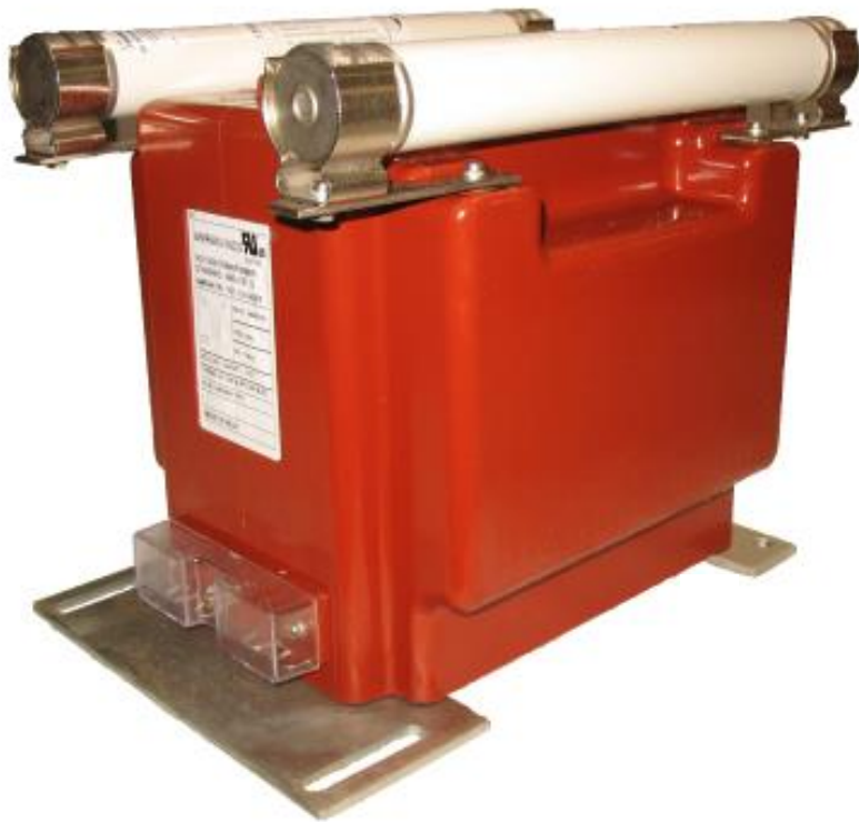
Model V21.1 – Medium Voltage Potential Transformer Maximum System Voltage 15.5 kV, BIL 110kV full wave
